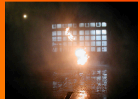
Above is 6.0MW Diesel spray fire getting extinguished within 12 seconds from Fogex system activation.
