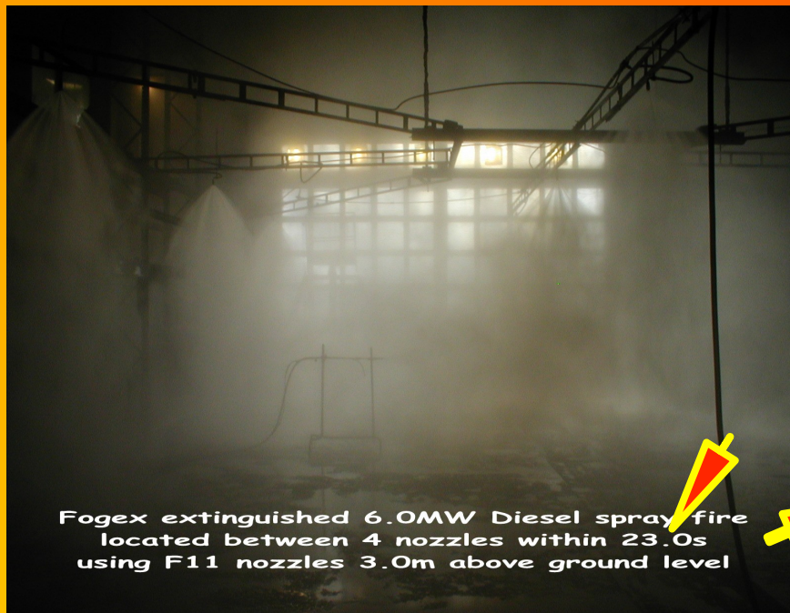
Above is 6.0MW Diesel spray fire approx. 3 seconds after Fogex has been activated.
