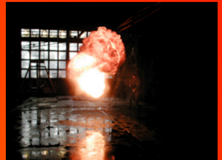
Above is a 6.0 MW Diesel spray fire moments after ignition
