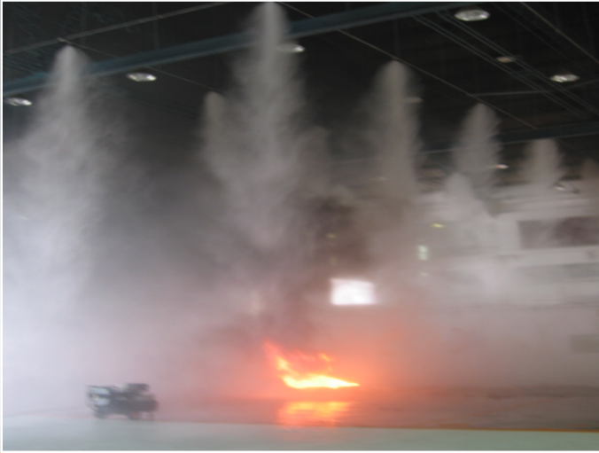
TAIWANESE AIR FORCE F-16 DUMMY IN HANGAR Fire Extinguished in Seconds
