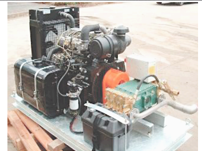
Diesel driven Pump unit
