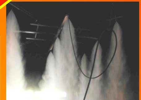
Above is a Fogex cold discharge test revealing very fine mist droplets with nozzles
